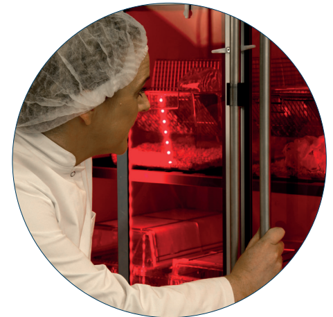
Red LED light is applied for easy inspection, when it is “night” and white LED light for simulation of “day” inside the ScanTainer
