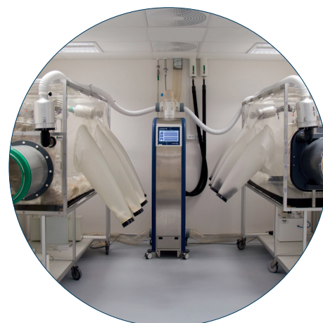
ScanClime supplying humidified/dehumidified air to isolators
